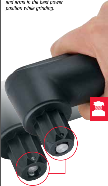
The patented locking mechanism features two stainless steel pins that automatically retract when the handle's full-length grab bar is squeezed, and extend when it is released for a solid, secure lock.
