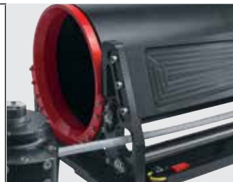
Hydraulic versions have an open-ended design to reduce weight.
