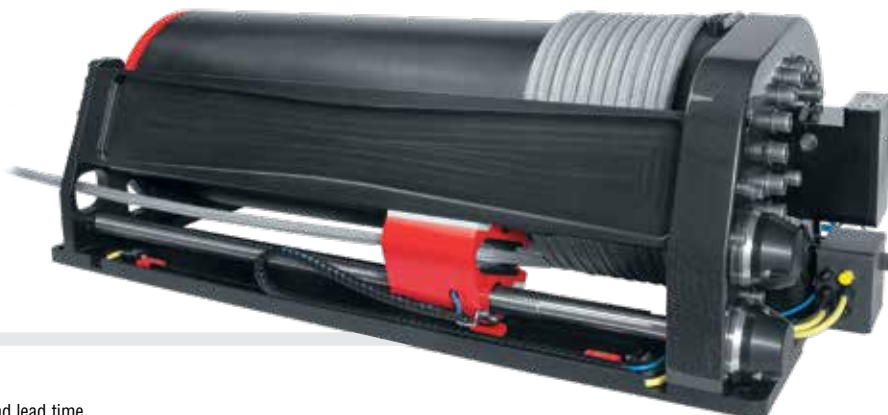
Two inner magnetic switches factory-set at the feeder's stroke limits prevent overtravel. Two outer fail-safe limit switches automatically engage the brake.
